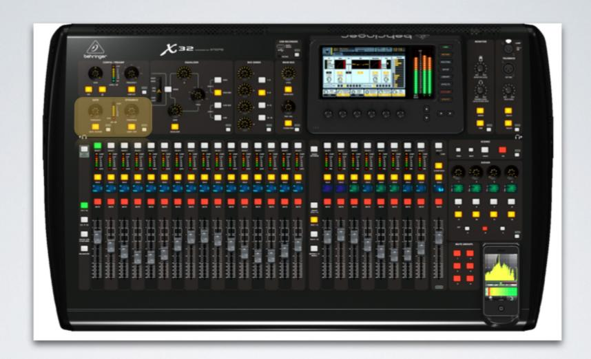
The signal now travels through the gate and dynamics highlighted above.
