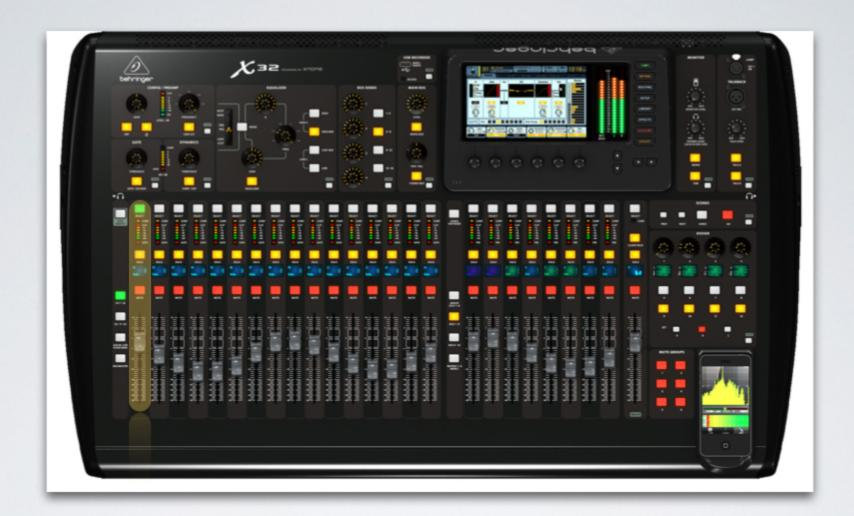
After the output sends we come to the Fader strip. The first button is the select button which associates the top left portion of the board to that channel. Next is a level meter, below that is the solo button for isolating channels for monitoring with headphones. The Scribble strip is completely digital and easily labeled, Mute is directly above the channel fader.
