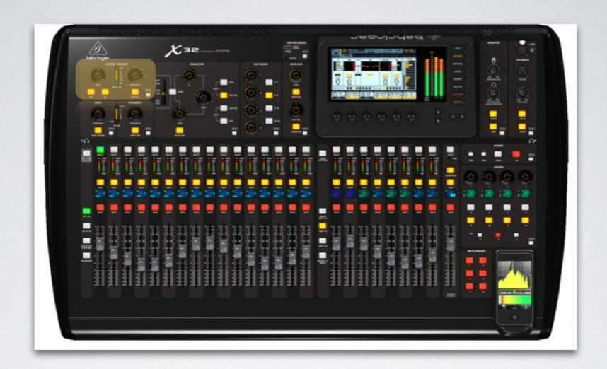
The highlighted area is the gain and low cut filter option.
